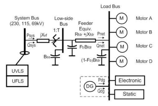
Figure 5.4.1: Composite Load Model Structure (CMPLDW/CMLD)
